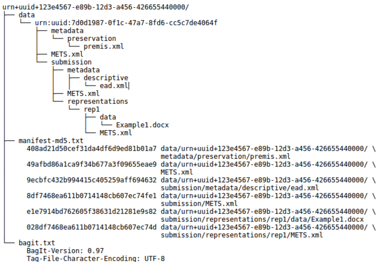
Figure 15: AIP in the data folder of a BagIt container.
