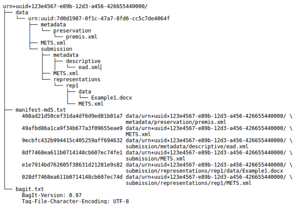
Figure 14: AIP content extracted from a TAR package.
